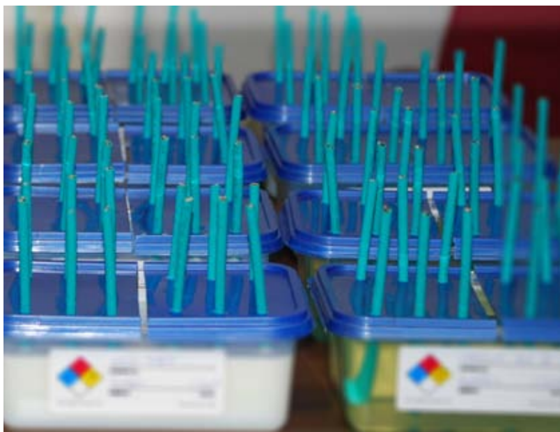
Chemical tests (affectionately nicknamed the “bean sprout tests”) being conducted to validate the resistance of the TPE (thermoplastic elastomer) cable jacket to chemicals commonly found in a heavy manufacturing environment such as cutting fluid, oil and robotic grease.
