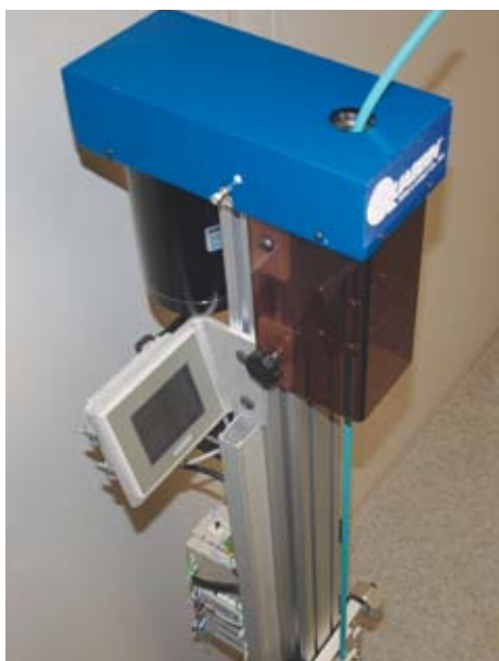
Torsion tests are performed on Quabbin 2 pair UTP industrial Ethernet cable and Quabbin 4 pair double shielded cable. This 34” test sample is subjected to a 360 degree twist per cycle (180° in each direction). Three Million cycles are completed on each design with no apparent physical degradation and the cable continues to exceed electrical performance specifications.
