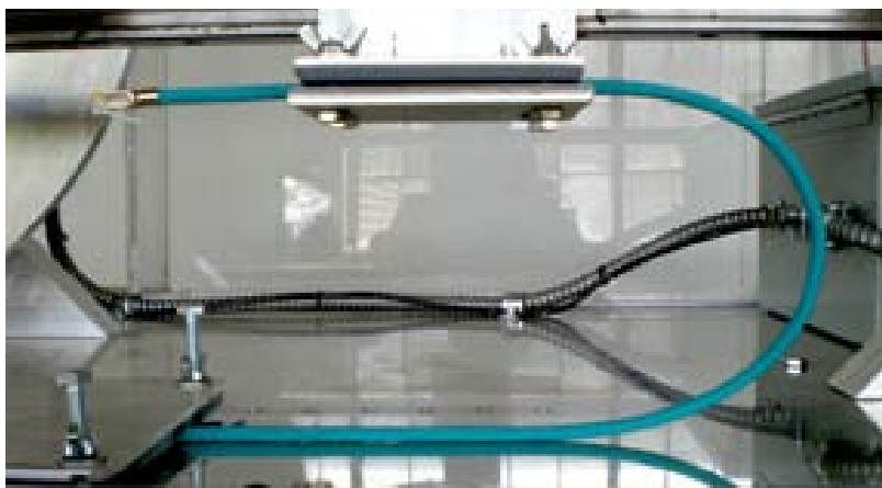
Rolling bend flex tester , below, showing a 4 pair, double shielded (foil & braid), DataMax® Extreme with ZHFR-PUR jacket being tested to 10 million cycles. Results were a cable with no physical damage that continued to surpass category 5e test parameters.
