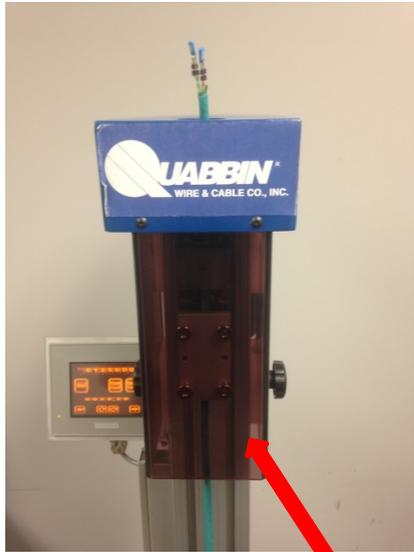
3. The rotation end could be dangerous and harmful so it is important to close the rotating top with the plastic shield
