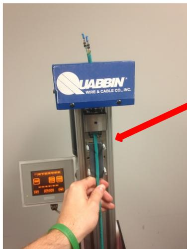
1. The cable is fed through the top hole. A short length of about 1 inch of cable is exposed at the rotating end to avoid unintended flexing of the cable as the rotation reversed.
