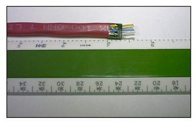
**Step 6** Slip the load bar outward toward the end of the cut leads. Stop the load bar just short of the immediate end. (**Note**: The purpose of the load bar is to "aim" the leads so that they enter the plug cavity precisely positioned to pass through to the correct pin positions.)
