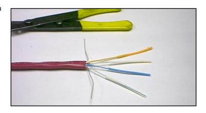
In either event, the removal process must be performed using a pull direction in a straight line with the cable's construction. If the pull direction is at an angle, the inner insulation is at risk.
