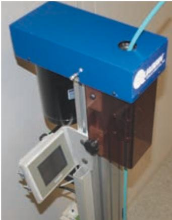
**Torsion tests** are performed on Quabbin 2 pair UTP industrial Ethernet cable and Quabbin 4 pair double shielded cable. This 34” test sample is subjected to a 360 degree twist per cycle (180° in each direction). Three million cycles are completed on each design with no apparent physical degradation and the cable continues to exceed electrical performance specifications.
