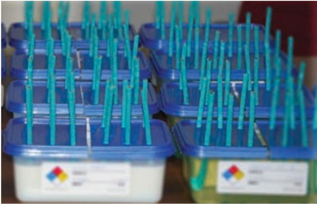
**Chemical tests** being conducted to validate the resistance of the TPE (thermoplastic elastomer) cable jacket to chemicals commonly found in a heavy manufacturing environment such as cutting fluid, oil and robotic grease.
