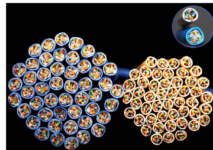
Figure 3: Comparison of 26 AWG and 28 AWG DataMax patch cable. DataMax Mini 6a F/UTP 28 AWG patch cable is 23% smaller in size, 38% smaller in cross-sectional area and 33% lighter than standard 26 AWG cable. Source: Quabbin Wire and Cable Co.
