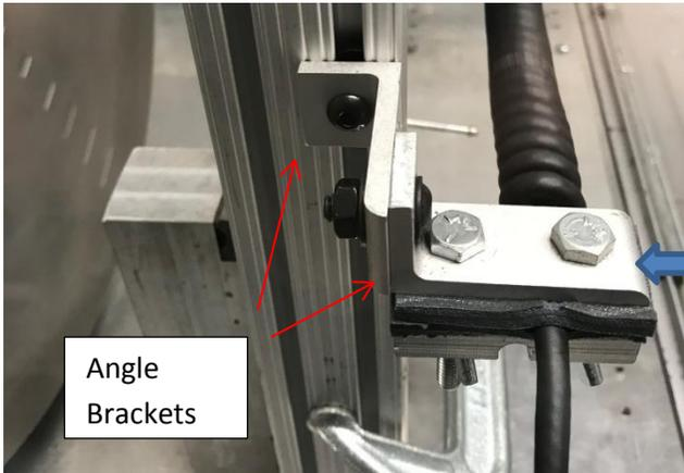
3. A slide nut is used to attach a small angle bracket to the 80-20 stock. The height should be adjusted to match the mount height at the other end of the track. A second angle bracket is attached to this bracket.
