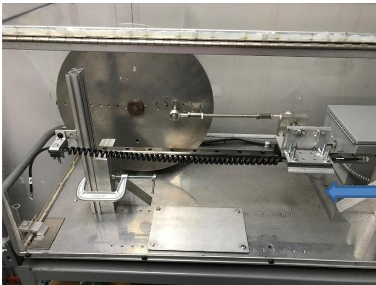
1. An overall view of the test setup can be seen to the left. The cable will be secured at either end, and positioned such that the coil will go from no extension to an extension of about 2x the static length.
