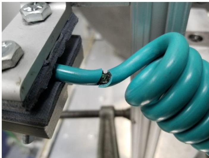
A cable dissection indicated that the brown pair was almost completely severed, and the other pairs showed some small signs of wear.
