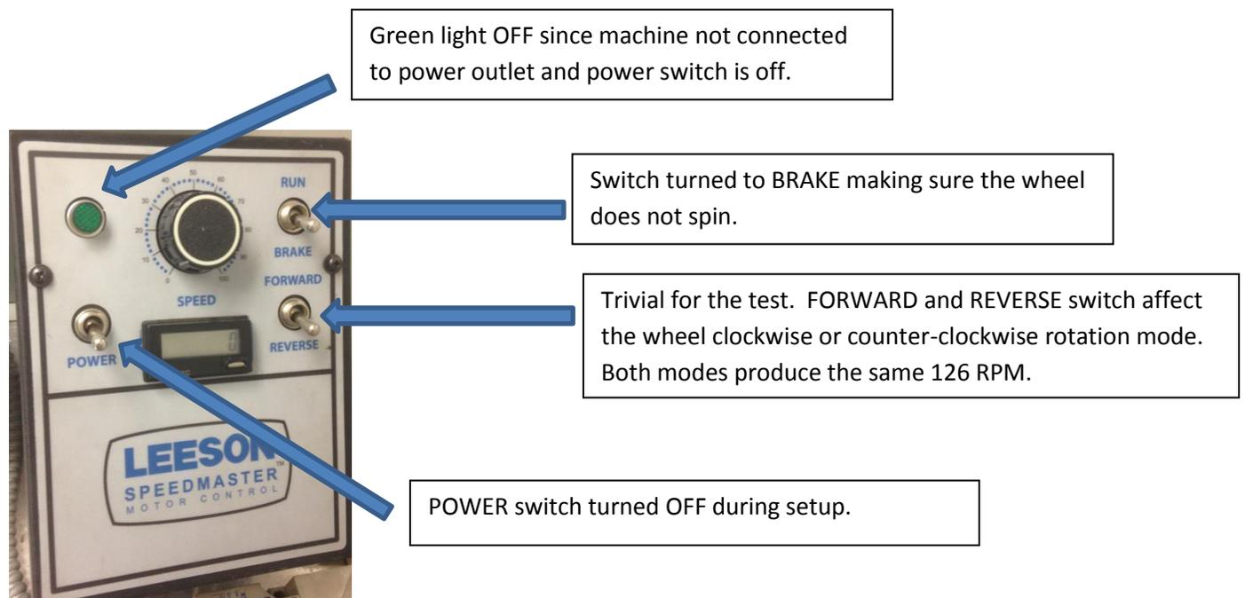
When machine is securely OFF, the cable setup can begin. The machine is capable of testing one or two cables at once. If 2 cables have a similar O.D., then it is possible to test them together. Prior to setting up the cables in the flex machine, pins and loads must be installed on both ends of the cables. The testing of the cable follows Quabbin standard procedures. Inserting the cable into the flex machine can begin once the cables are pinned or connectorized.
