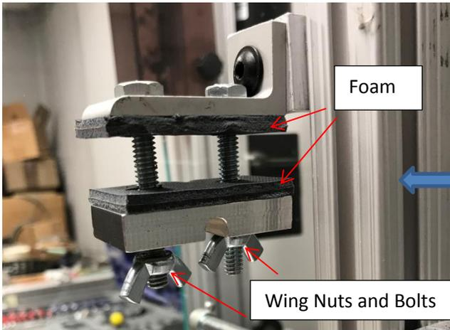
4. A small piece of adhesive backed foam is used to protect the cable on the lower angle bracket. A straight piece of aluminum is attached to the 2<sup>nd</sup> angle bracket using bolts and wingnuts, again adhesive backed foam is used to protect the cable. The wing nuts should be tightened enough to secure the cable but not overtightened.
