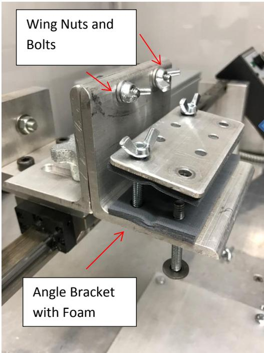
6. A second large angle bracket is mounted back to back with the one from above, two bolts and wing nuts can be used to attach the brackets. A piece of adhesive backed foam is attached to the flat part of the bracket.
