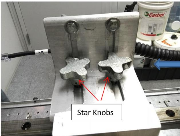
5. Star knobs are used to secure a larger angle bracket to the flex tester base. The position of this bracket can be adjusted to keep it in line with the other end of the test fixture.
