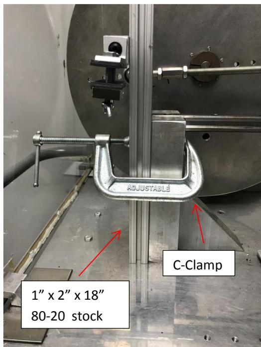
2. A c-clamp was used to secure a piece of 1" x 2" x 18" 80-20 stock. Ensure that the position of the c-clamp doesn't interfere with the motion of the flex tester.
