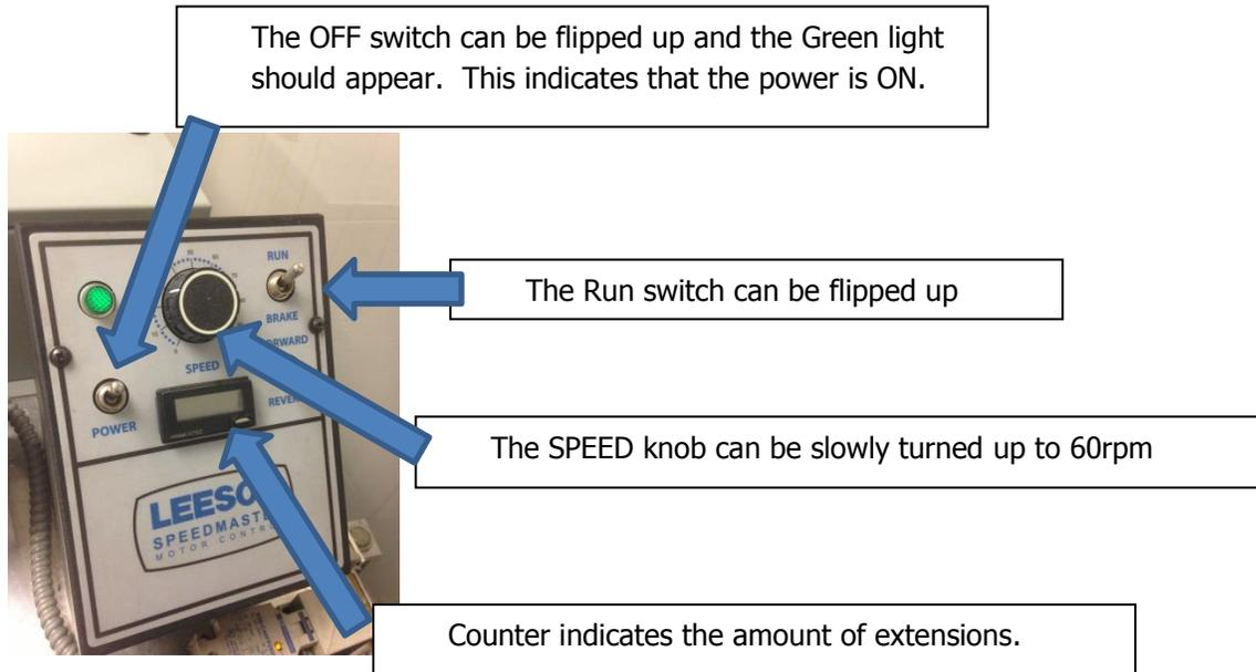
When the machine begins to run and cycle the coil cord, the access door is to be shut and locked for safety.
