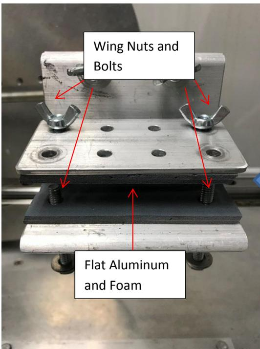
7. A flat piece of aluminum is attached to the angle bracket using 4 bolts and wing nuts. A piece of adhesive backed foam is used to protect the cable. Route the cable through the center of the bracket. Tighten the wing nuts just enough to hold the cable but not so tight that the cable is deformed or damaged.
